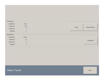
Press the Dump/Top-Up Button to access the Hopper Dump/Top-Up Menu.
