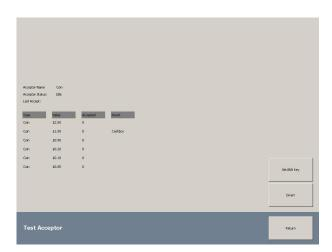
To test the Coin Validator, press the Coin Acceptor Button. This menu allows you to test the Coin mechanism, informs you of the operational status and allows you to test the Coin Divert pressing the Divert Button.
