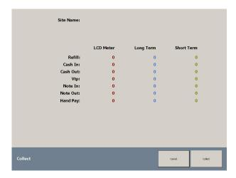
Once in the "Collect" menu you can view all the Long and short term meters. To perform a collection, press the "collect" button.
