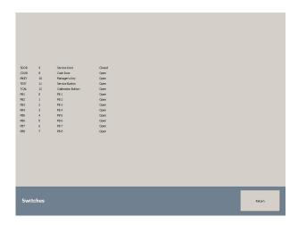
Press the Switches Button to open the Switch Test Menu. Here you can test the cabinet/play panel switches to ensure they are functioning correctly by pressing the buttons, the screen will show open/closed when buttons are pressed.
