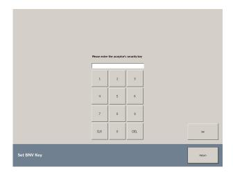
Press the Set BNV Key Button to set the security code for the Note Validator.
