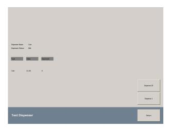
Press the Coin Dispenser Button to access the Hopper Test Menu. This menu allows you to test the payout of the Hopper by paying out 1 x Coin or 20 x Coins, this is done by pressing the corresponding Dispense 1 or Dispense 20 Button.
